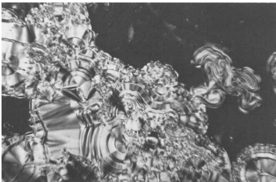
FIGURES 11, 12 and 13. Formation of S_x phase from nematic phase at 87.6°C. See Color Plate I.
